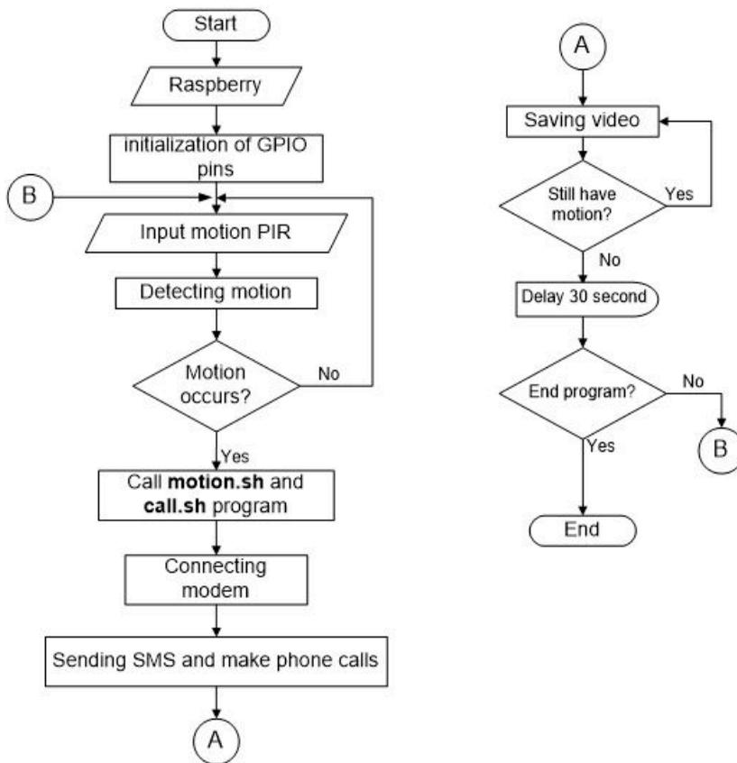
Figure 3. Flowchart of Main Program on Raspberry
