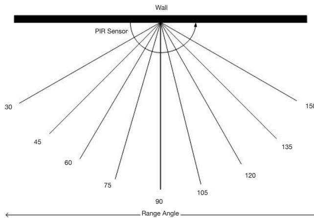
Figure 6. PIR sensor test scenarios from various angles
