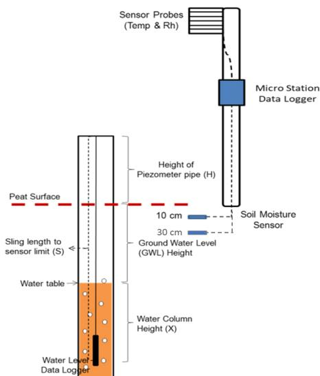
Figure 1. The design of groundwater level and peat water content measurement
