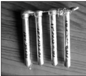
Figure 2. Casting used for Tensile test specimen
