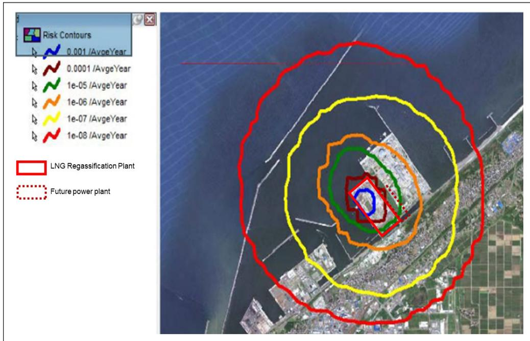
Figure 8. INPEX LNG regasification terminal - LSIR contours
