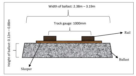
Figure 8. The main component of track with the range of dimension at site
