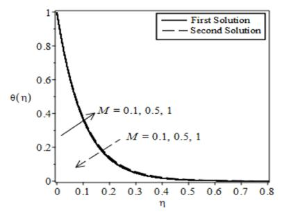
*Figure 11.* Temperature profiles for various values of *M* for magnetite at  $\lambda = 0.5$ .
