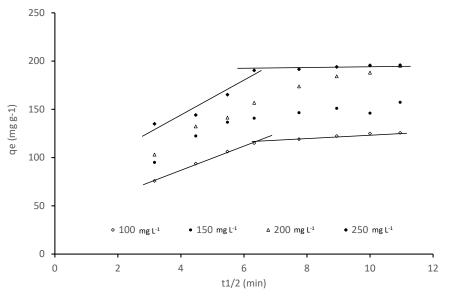
Figure 9. The IPD modeling of Pb uptake by AC-4 at varied concentrations (Initial pH = 4; ads. dosage = 0.13 g)
