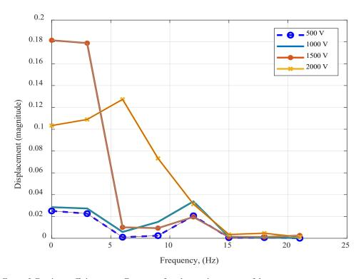
Figure 5. Fourier coefficient versus Frequency for a harmonic response of the actuator
