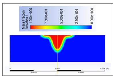
Figure 4. Weld pool shape for test run-1
