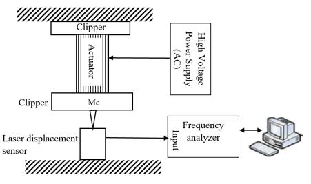
Figure 3. Harmonic electrical input testing
