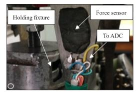
Figure 2. The attached tangential force sensor
