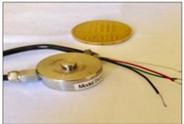
Figure 3. The employed load cell sensor
