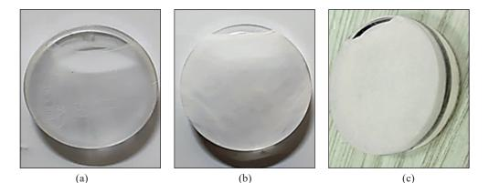
*Figure 1*. Attachment of membrane to blood feeder reservoir a) Parafilm-M; b) PTFE tape; c) Collagen sausage casing. Rubber band was used to attach collagen sausage casing to blood feeder reservoir.
