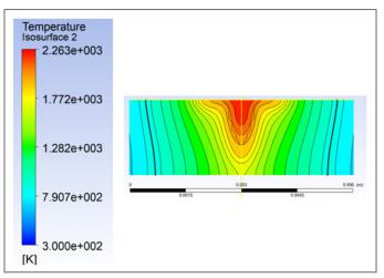
Figure 9. Temperature distribution for test run-2 (pulse width= 8 ms; welding speed= 1.5 mm/s)
