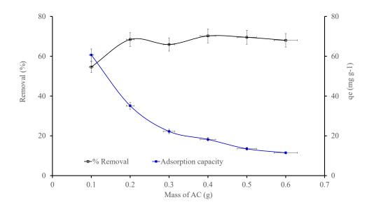
*Figure 5*. Extent of Pb(II) ion uptake and adsorption capacity of AC-4 at different adsorbent dosage. (Pb(II) =  $50 \text{ mg } \text{L}^{-1}$ ; Solution pH = 4)
