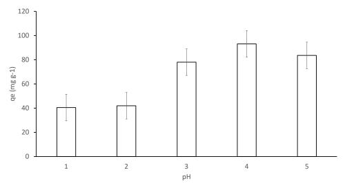
*Figure 7*. Sequestration of Pb(II) on AC-4 at different pH of the Pb(II) solution (Condition: 0.13 g AC-4; 80 mg L<sup>-1</sup> Pb(II))
