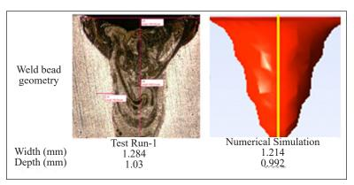
Figure 5. Comparison of simulated weld bead geometry with test run-1
