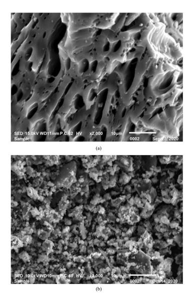
Figure 1. SEM images of (a) CAC and (b) CS-NMAC at 2000× magnification at 10.0 kV
