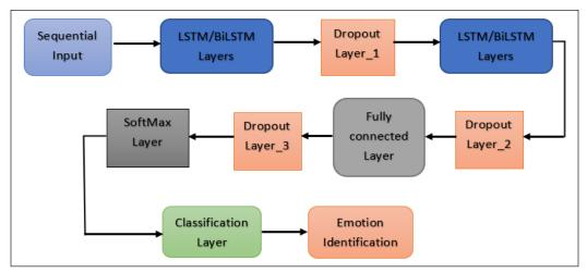
Figure 3. Proposed DNN design layer architecture
