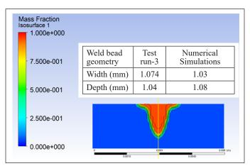
Figure 10. Weld pool shape for pulse width 7 ms and welding speed 1.0 mm/s
