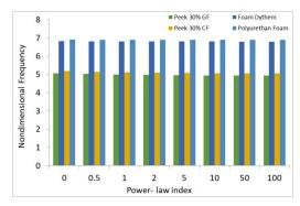
*Figure 9.* Results of the natural frequency at Beta =0.1, for various porous metals at FG core height 10 mm, and face thickness 2.5 mm
