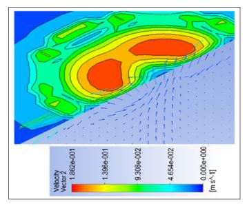
Figure 7. Velocity contour plot in the weld pool (test run-1)
