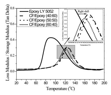
Figure 5. Tan Delta of carbon fibre composites
