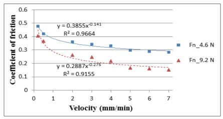
Figure 7. Coefficient of friction vs velocity
