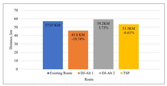
*Figure 14.* Comparison chart of existing and alternative routes from Prai industrial area to Ampang Jajar Waste Transfer Station.
