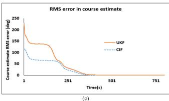
Figure 6. RMS error for Scenario 5: (a) Range estimate; (b) Speed estimate; and (c) Course estimate
