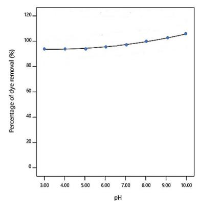
*Figure 4*. Percentage removal (%) of Rhodamine 6G by CS-NMAC in batch adsorption reaction at 27 °C, 150 rpm and 0.05 g CS-NMAC according to pH.
