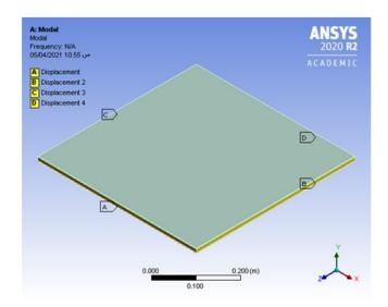
Figure 4. FGM Sandwich plate
