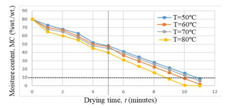
Figure 8. Moisture content against time with different temperature of hot air feed
