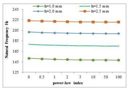
*Figure 10.* Results of the natural frequency at Beta =0.1, for various face sheet thicknesses with FGM core height 5 mm
