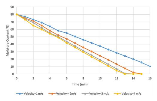
Figure 4. Moisture content of sago bagasse at different inlet velocities of hot gas
