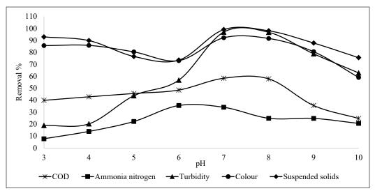
Figure 5. Dual coagulant of PAC (3,500 mg/L) and MEP (250 mg/L) at varied pH 3.0-10.0
