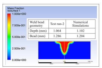
Figure 8. Weld pool shape for pulse width 8 ms and welding speed 1.5 mm/s
