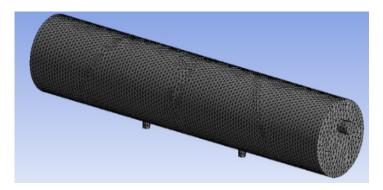
Figure 2. 3D Meshing of the FBD model
