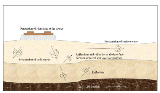
Figure 2. Propagation movement for ground vibration (Persson, 2016)
