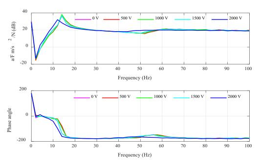
*Figure 4.* Acceleration per unit force for different DC voltage supply at mass = 0 (pre-stretch due to clipper mass of 105 g)
