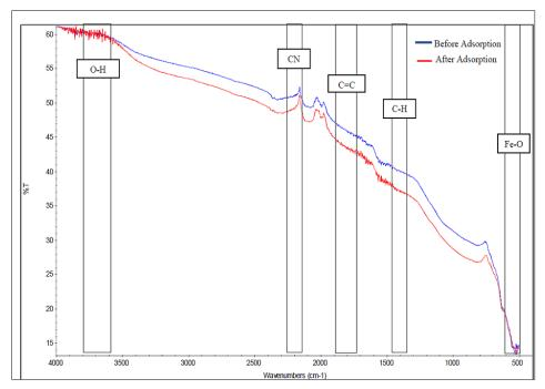
Figure 8. FTIR spectra of CS-NMAC before and after adsorption of Rhodamine 6G dye
