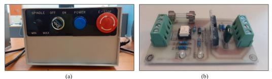
Figure 4. INNER Microchip Driver Interface v.2.0: (a) Control box; and (b) Driver board
