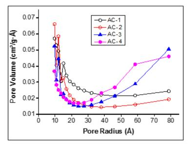
Figure 2. Pore size distribution of the prepared ACs
