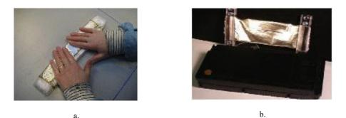
*Figure 1.* (a) A rolled multilayer DEAP composite pressed to form a flat structure. (b) A photograph of the final assembly of Poly Power flat DEAP actuator (Rahimullah Sarban, 2011)
