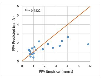
Figure 13. Predicted PPV versus empirical PPV
