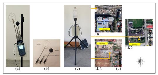
*Figure 3*. The instruments used in the present study: (a) Delta Ohm Thermocouple Infrared Thermometer; (b) The instruments probe; (c) Seven Elements Integrated Weather Sensor WTS700; (d) Seven Elements Integrated Weather Sensor WTS700 location for all three case study lockups
