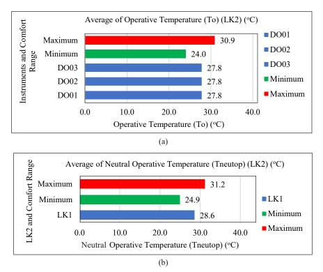
Figure 7. Summaries of the (a) operative temperature and (b) neutral operative temperature prediction for LK2
