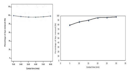
*Figure 3*. Percentage removal (%) of Rhodamine 6G by CS-NMAC in batch adsorption reaction at  $27^{\circ}$ C, 150 rpm and 0.05 g CS-NMAC according to (a) 15–60 min and (b) 5–30 min of contact time.
