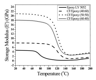
Figure 4. The storage modulus of carbon fibre composites
