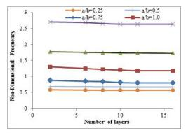
Figure 13. The natural frequency for different number of layers of FGM rectangular plate gradient index k = 2 and Beta=0.1
