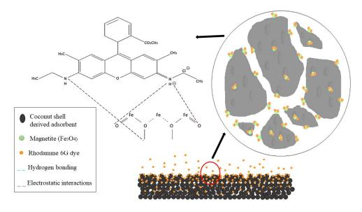
Figure 7. Chemisorption between Rhodamine 6G and surface of CS-NMAC
