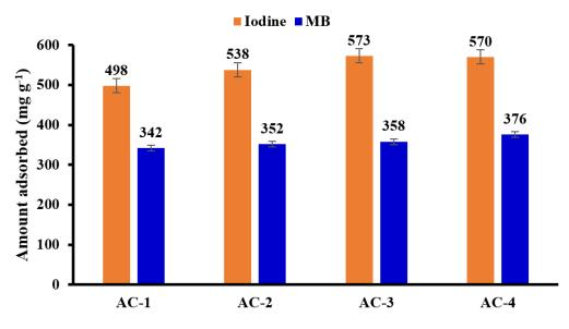
Figure 3. Iodine and MB uptake by various AC samples
