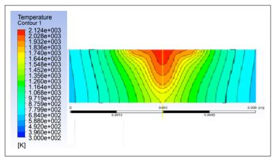
Figure 6. Temperature distribution (test run-1: pulse width= 9 ms; welding speed=2 mm/s)
