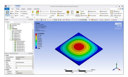
Figure 6. View of Modal Analysis of FGM sandwich plate
