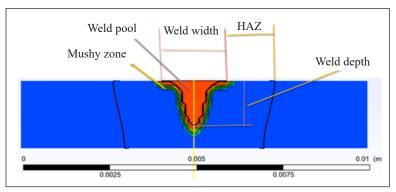
Weld Bead Profiles of Ti-6Al-4V alloy using Laser Beam Welding
