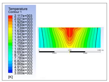
Figure 11. Temperature distribution for test run-3 (pulse width= 7 ms; welding speed= 1.0 mm/s)
