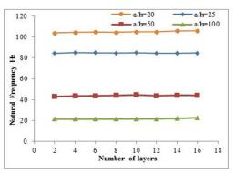
*Figure 14.* The natural frequency for different number of layers of FGM square plate with gradient index k = 2 and Beta=0.1
