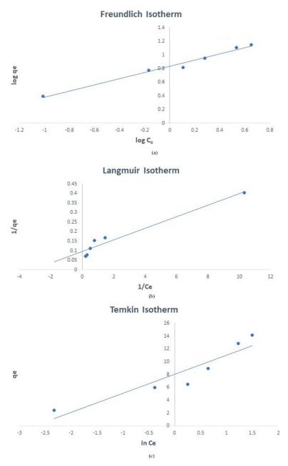
*Figure 5*. Graphs depicting the removal of Rhodamine 6G in aqueous solution by CS-NMAC at 27°C; 5, 10, 10, 15, 20 and 25 mg/L initial concentration (Co); 0.05 g adsorbent dose; 150 rpm agitation rate; and 14.33 min contact time: (a) Langmuir isotherm, (b) Freundlich isotherm and (c) Temkin isotherm.
