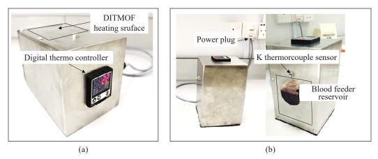
*Figure 2*. Digital Thermo Mosquito Blood Feeder (DITMOF) in: (a) horizontal position; and (b) vertical position (feeding position)
