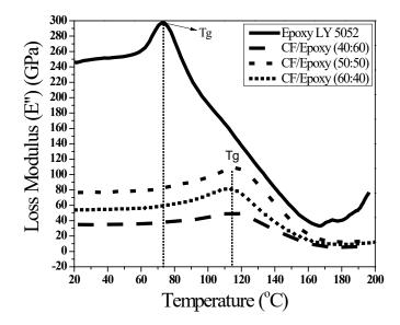
Figure 3. Loss modulus vs temperature (°C) of carbon fibres composites
