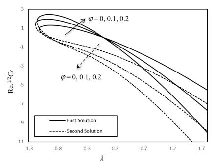
*Figure 6.* Effects of  $\varphi$  on skin friction coefficient with *M*=0.5 and *S* = 2.
