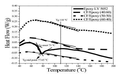
Figure 2. Heat flow vs transition temperature of carbon fibre composites
