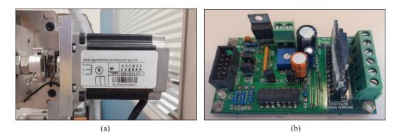
Figure 3. Unipolar Microstepping Board: (a) Stepping motor; and (b) Microstepping board
