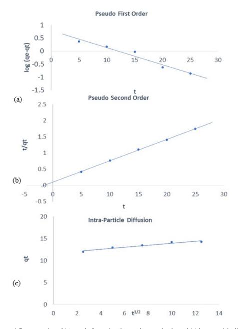
*Figure 6.* Representation of (a) pseudo-first order, (b) pseudo-second order and (c) intra- particle diffusion plots for Rhodamine 6G adsorption into CS-NMAC at 27 °C, 150 rpm agitation, 26.12 mg/L dye concentration and adsorbent dose of 0.05 g.
