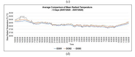
*Figure 8*. Statistical summaries of the average comparison indoor and outdoor measurements for LK3: (a) Air temperature; (b) Air speed; (c) Relative humidity; (d) Mean radiant temperature
