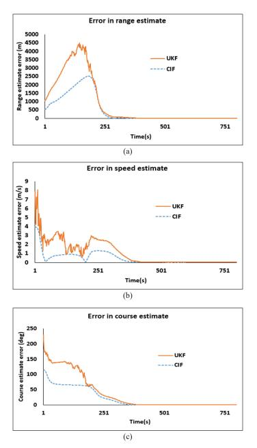
Figure 5. Error for Scenario 5: (a)Range estimate; (b) Speed estimate; and (c) Course estimate
