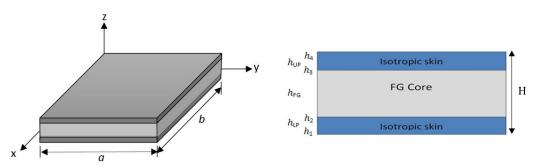
Figure 3. Geometry configurations of FGM porous sandwich plate
