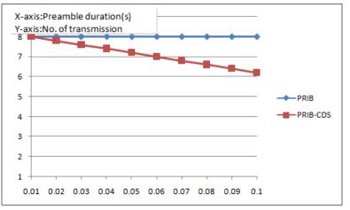
Figure 3. Number of transmissions with different preamble duration
