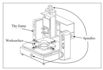
Figure 2. Mini CNC ceramic machine structure
