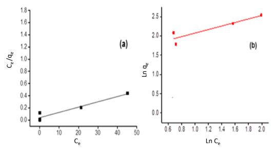
Figure 8. Adsorption isotherm of Pb(II) linearized according to (a) Langmuir (b) Freundlich
