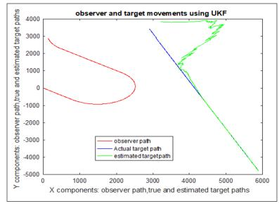
Figure 4. Observer and target movements using UKF
