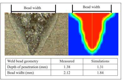
Figure 2. Comparison of simulated weld bead geometry with the test result (Jiang et al., 2019)
