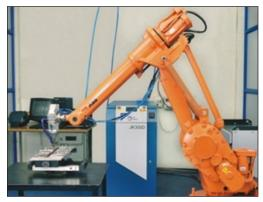
*Figure 3.* Experimental set-up for pulsated LBW of Ti-6Al-4V alloy
