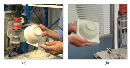
Figure 9. Outcome of ceramic work piece milling bowls: (a) Clay bowl; and (b) Plaster bowl
