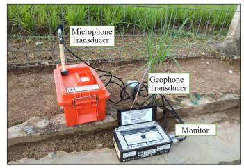
Figure 9. Mini-Seis installed at the studied site
