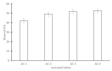
*Figure 4.* Removal of Pb by activated carbon prepared at different activation time (Condition: 50 mg  $L^{-1}$  of Pb(II); 0.1 g of AC, pH of solution = 4)
