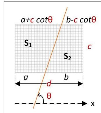
Figure 6. Soil proportion of two-layer vertical soil
