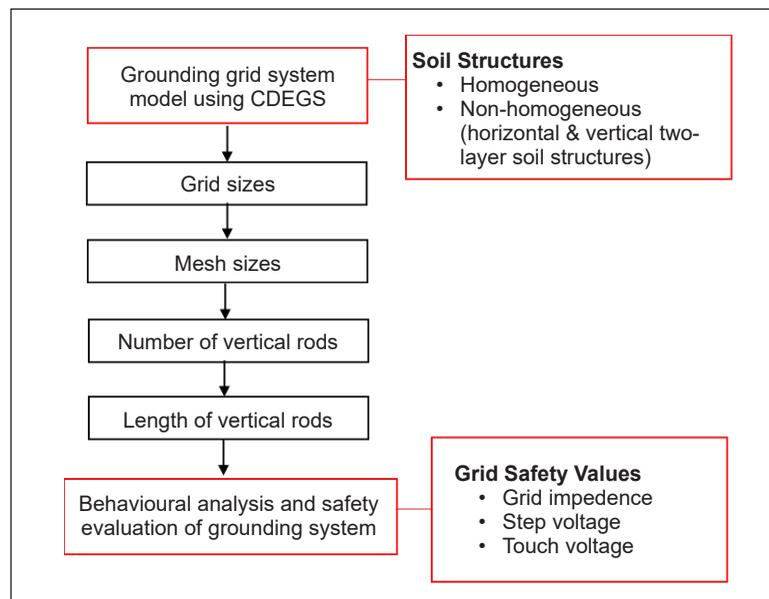
Figure 2. Methodology of grounding system design analysis
