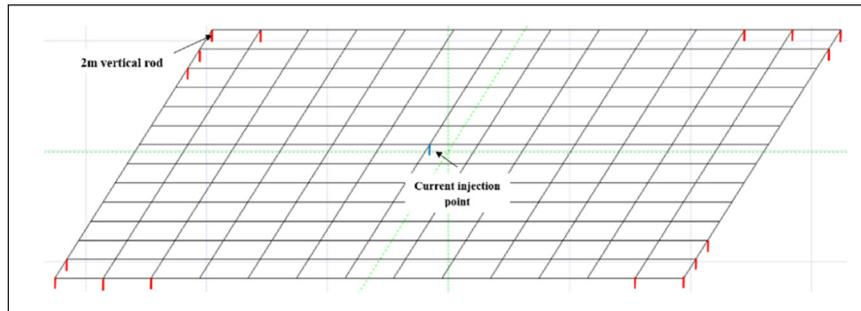
Figure 3. The grounding grid comprises 16 vertical rods attached
