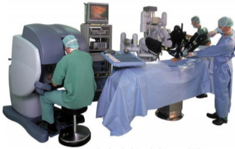
Figure 1. The da Vinci robotic surgery system
