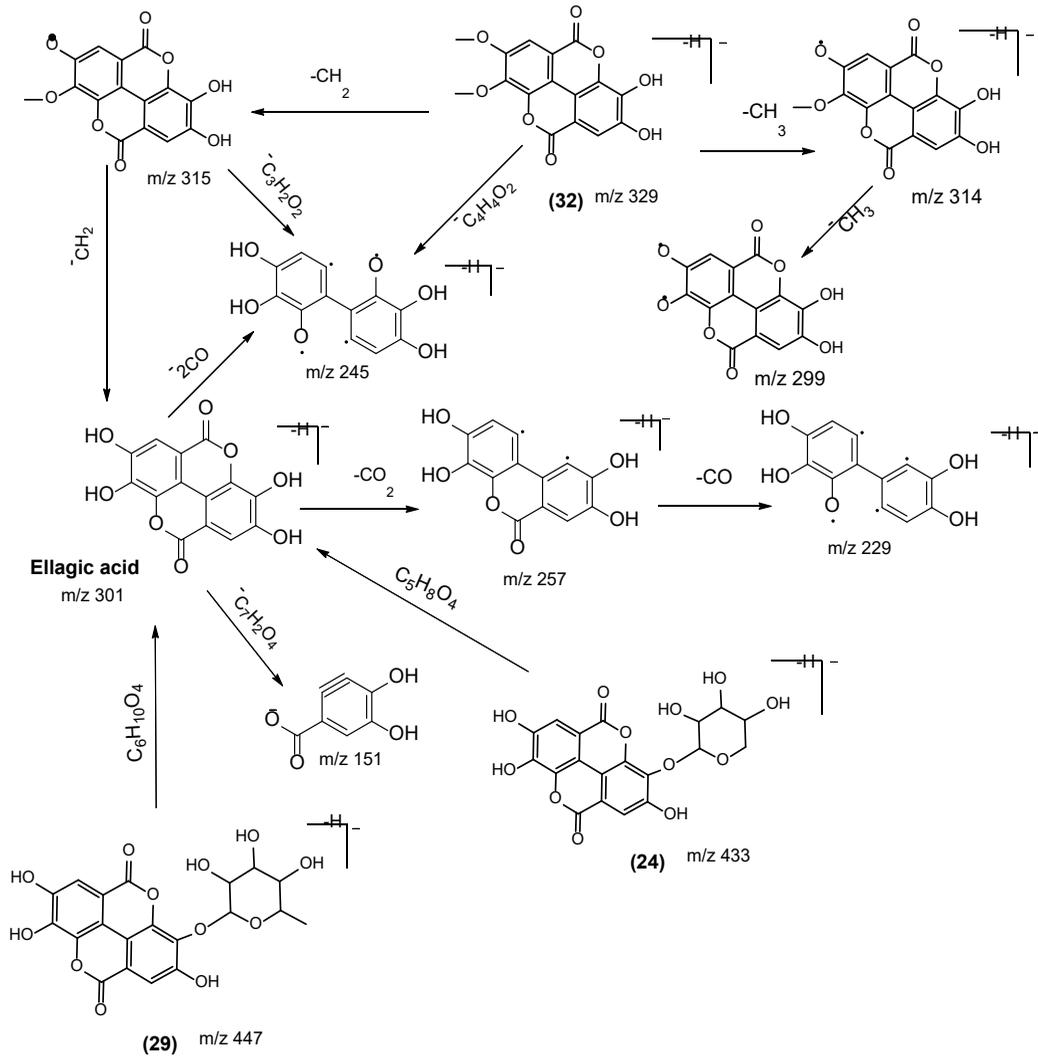
SD4. Proposed fragmentation pattern of ellagic acid pentoside **24**, ellagic acid deoxyhexoside **29** and 2,3-di-O-methylellagic acid **32**
